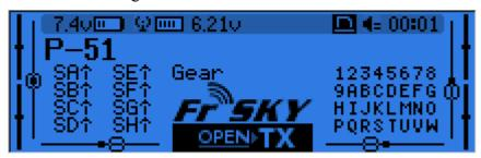
The last view is a channel monitor showing the servo outputs for all 32 channels (+/- change page). If channel names are defined on the SERVOS page, they will show up here instead of the numbers for convenience.
