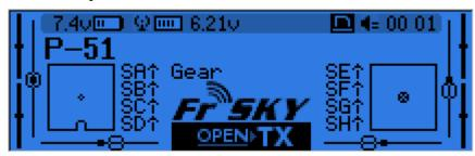
The third shows again the physical switches on the left, and the states of the 32 custom (logic) switches on the right.
