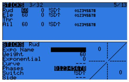
As many lines as required can be assigned to each stick (LONG press ENTER brings up a popup menu), and again the first one that has its switch on (starting from the top) will be the active one. This is commonly used to create dual, triple,... rates. A name can be defined for each entry, as well as the rate and exponential ratio. A curve (built-in or custom) can also be used instead of the "simple" exponential function.
