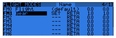
8 flight modes plus the default one are available for use. Each of them can be named, has a selectable activation switch (physical or logical), a trim selection array (R, E, T, A when shown mean the mode has its own trim setting for that control, but each can be changed to a number from 0 to 9 and thus use the same value as the specified mode), and slow up/down parameters for smooth transitions between modes.
