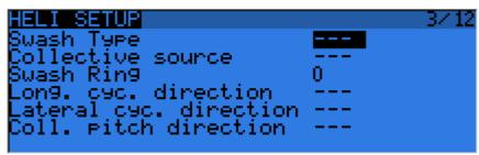
The inputs of this mixer are the Ail and Ele sticks, plus the virtual channel selected in "Collective source". This channel would see entries added on the MIXER page for one or more pitch curves.
