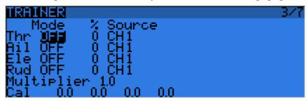
This page allows you to configure the trainer function for "master" use (make sure the Trainer mode in model settings is set to Master). For each of the 4 main functions you will be able to set the mode (OFF, += for Add, := for Replace), ratio and input channel.
