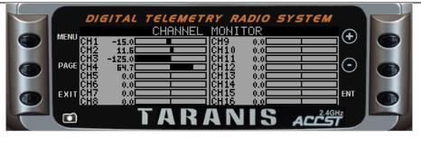
• [Short-Press MINUS ( -) or PLUS (+) buttons - to page down or up between CH1-CH16 and CH17-CH32 channel lineups]
